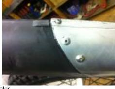
Fit both front pipe & silencer with new o-rings and silicone sealer. Also check that the middle-box brackets have no cracks....re-weld / repair if necessary.
